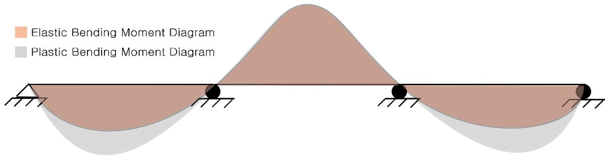
Fig. 2 Difference between Elastic theory and Plastic theory bending diagram
