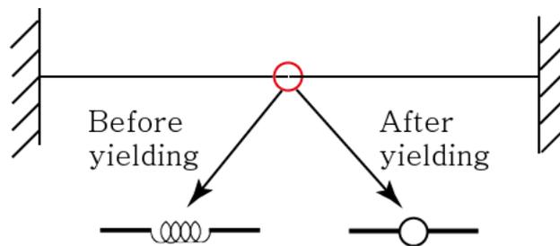
Fig. 1 Implementation of rotational spring elements
